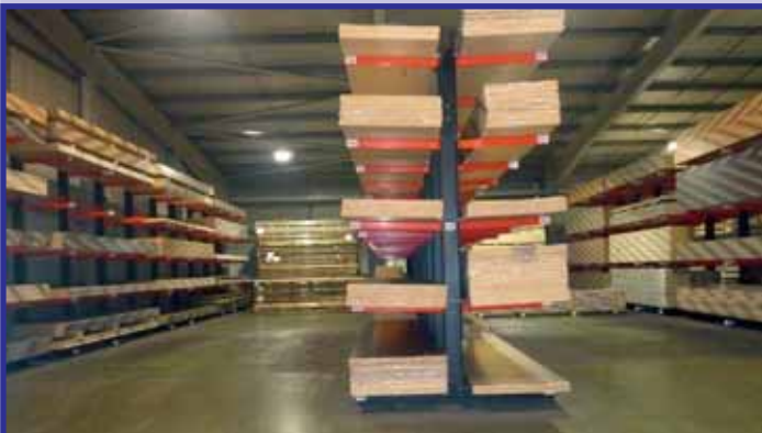
Cantilever racking for the storage of kitchen worktops.
